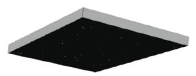
Kinetics Drop-In Panels are manufactured with 2" of 3 lb. density acoustic fiberglass for a greater than 1.0 noise reduction coefficient. These panels have unfinished square edges and are intended to be used in standard "T bar" or "grid" ceiling configurations, and have the preferred non-glare, matte black finish.
