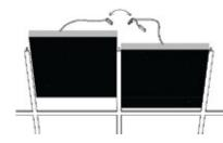
Connect a Jumper Cable to the first panel and connect it to the next panel. Up to 50 Kinetics Panels can be connected together in any configuration. If
