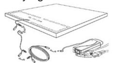
Connect the first panel to the Leader Cable. Inspect the front of the panel to see that the stars are illuminated.
