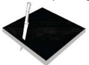
If necessary, cut the border with knife. Make sure to cut the Drop-In Panel from the face side along the marked lines. Make sure to make your cuts straight up and down and not at an angle.
