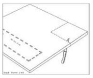
Caution: Each Kinetics Panel has a "No Cut Out Zone," if necessary, rotate the panel in order to avoid the "No Cut Zone."
